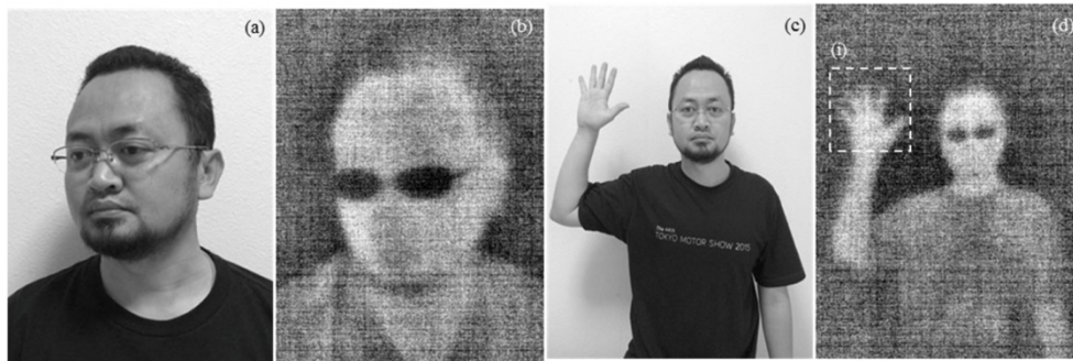
Fig. 17. Visible light and night vision images at different distances; (a)-(b) 400 mm and (c)-(d) 2 m, and rectangle (i) showing image aberration.
